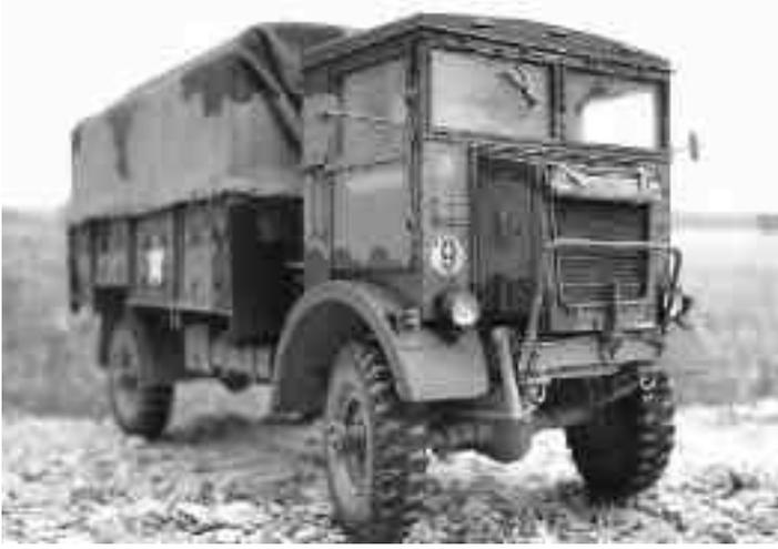
*Typical of a British Army three tonner but not as smoothly contoured as the ubiquitous Bedford QL. Note the substantial but somewhat vulnerable steering drop arm of a K5.*
